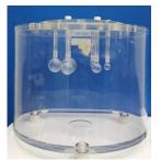
Figure 2. A NEMA body phantom with six spheres varying in sizes.
